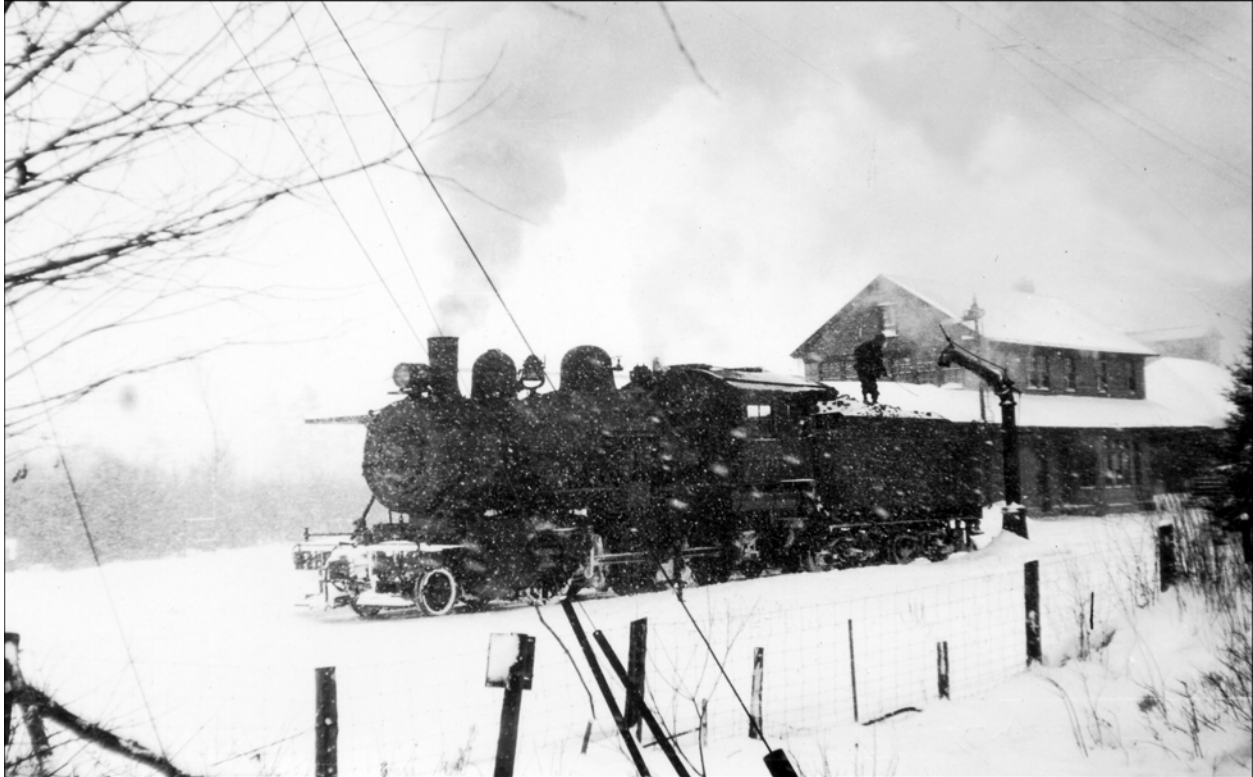
On a cold and snowy day at Cazenovia, one of the Chenango’s Moguls takes on water. That’s the final depot beyond the water standpipe.
